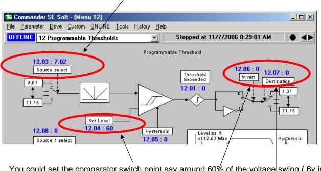
You could set the comparator switch point say around 60% of the voltage swing (6v in our case)
