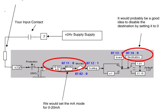
You could check to see if your input is working by observing parameter #7.02. It should be about 0.0 when your switch is open and about 100.0 when closed.
